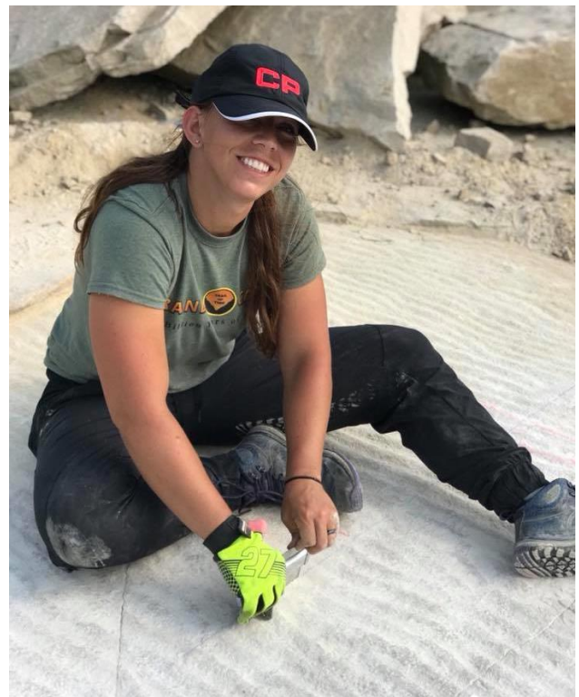
Jesse Dalle using a molding gauge to 'collect' ripples on a 500 million year old sandstone surface. The molding gauge produced a facsimile of a few ripples and this was traced onto roll paper and repeated until an entire exposed surface was replicated in cross section on paper.
